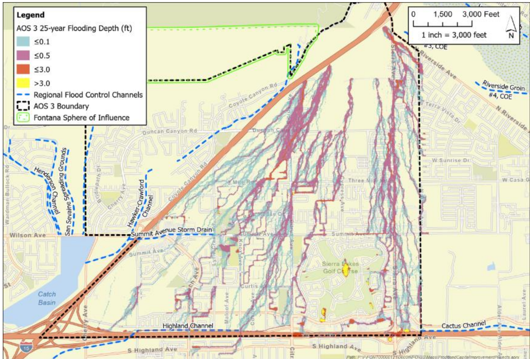
Figure 3-15. Existing Conditions 25-year Flooding in AOS 3
