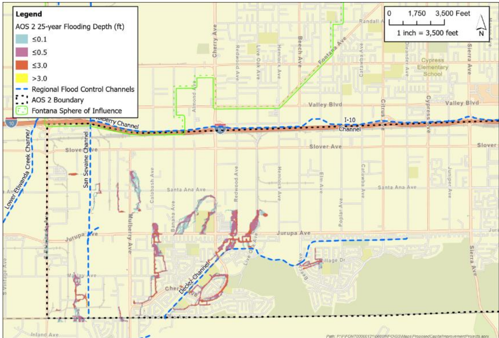
Figure 3-14. Existing Conditions 25-year Flooding in AOS 2
