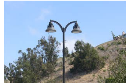
Figure 44. Hooded light fixture directs light downward.
