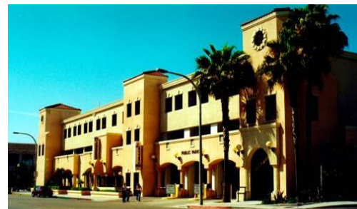
Figure 77. Horizontal and vertical articulation breaks up parking structure elevation.
