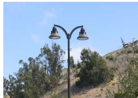
Figure 44. Hooded light fixture directs light downward.
