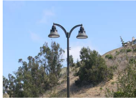
Figure 44. Hooded light fixture directs light downward.
