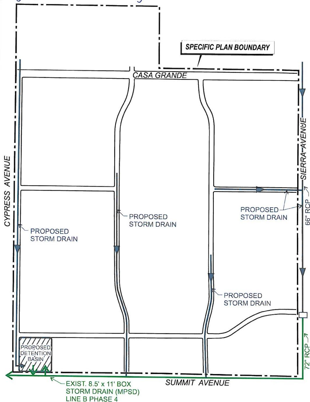
◆ Figure 5.3 Backbone Storm Drain System Condition C
